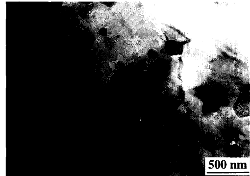
Fig. 3. Typical TEM microstructure of the \text{Al}_2\text{O}_3/10 wt% Ni-Co composite prepared by process B. Sintering condition was 1450^\circ\text{C} and 30 MPa for 1 h.
