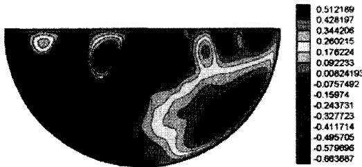
Fig. 7. Turbulent Mean flow Streamlines for Ra' = 7 \times 10^{14} and Pr = 8.3
