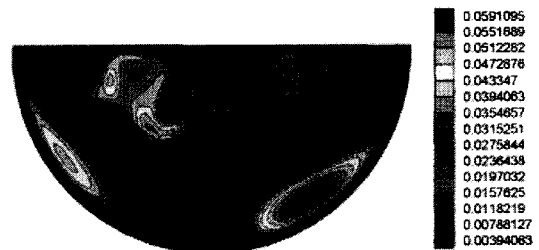
Fig. 10. Turbulent Viscosity for Ra' = 7 \times 10^{14} and Pr = 8.3
