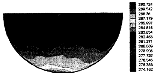
Fig. 9. Temperature Field for Ra' = 7 \times 10^{14} and Pr = 8.3
