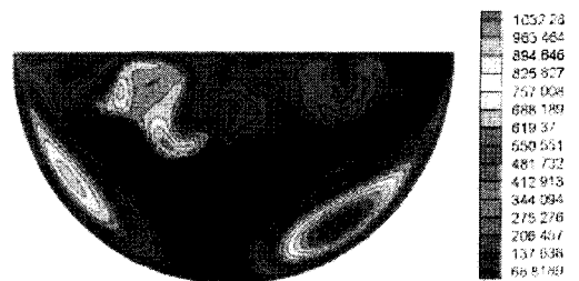
Fig. 13. Turbulence Reynolds Number for Ra' = 7 \times 10^{14} and Pr = 8.3
