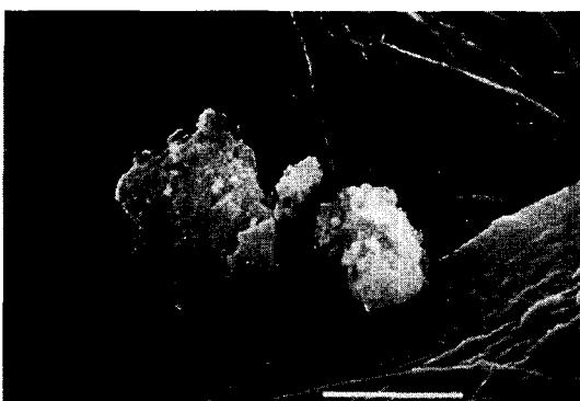
Fig. 10 (c). SEM of uncured rosin sized sheet surface with rosin emulsion coagulated for 72 hours with  $\text{Na}_2\text{SO}_4$  at 60°C.
