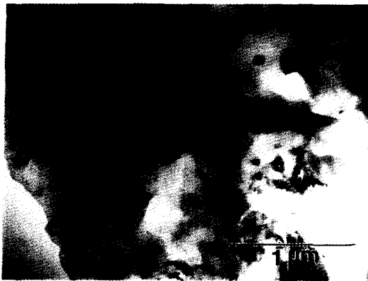
Fig. 4. TEM bright field images of Al-10%Ti-4%Fe extruded bar used for grain size measurement.
