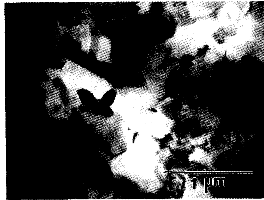
Fig. 7. Micrographs of Al-10%Ti-4%Fe sample after tensile test at 600°C.
