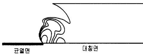
Fig. 8 Von Mises stress contour using bicharacteristic method
