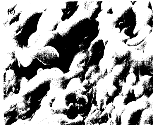
Fig. 6. SEM photographs to biodegradational behavior of PVA/Chitosan blends films (a) outer surface before bury, (b) after 7days and (c) 20days.
