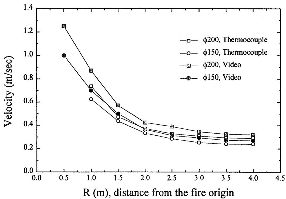
Fig 5. The smoke front speeds
