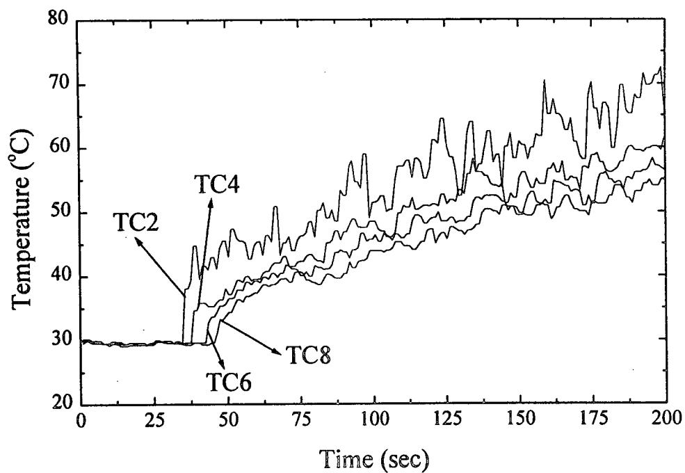
Fig 4. The smoke temperature change
