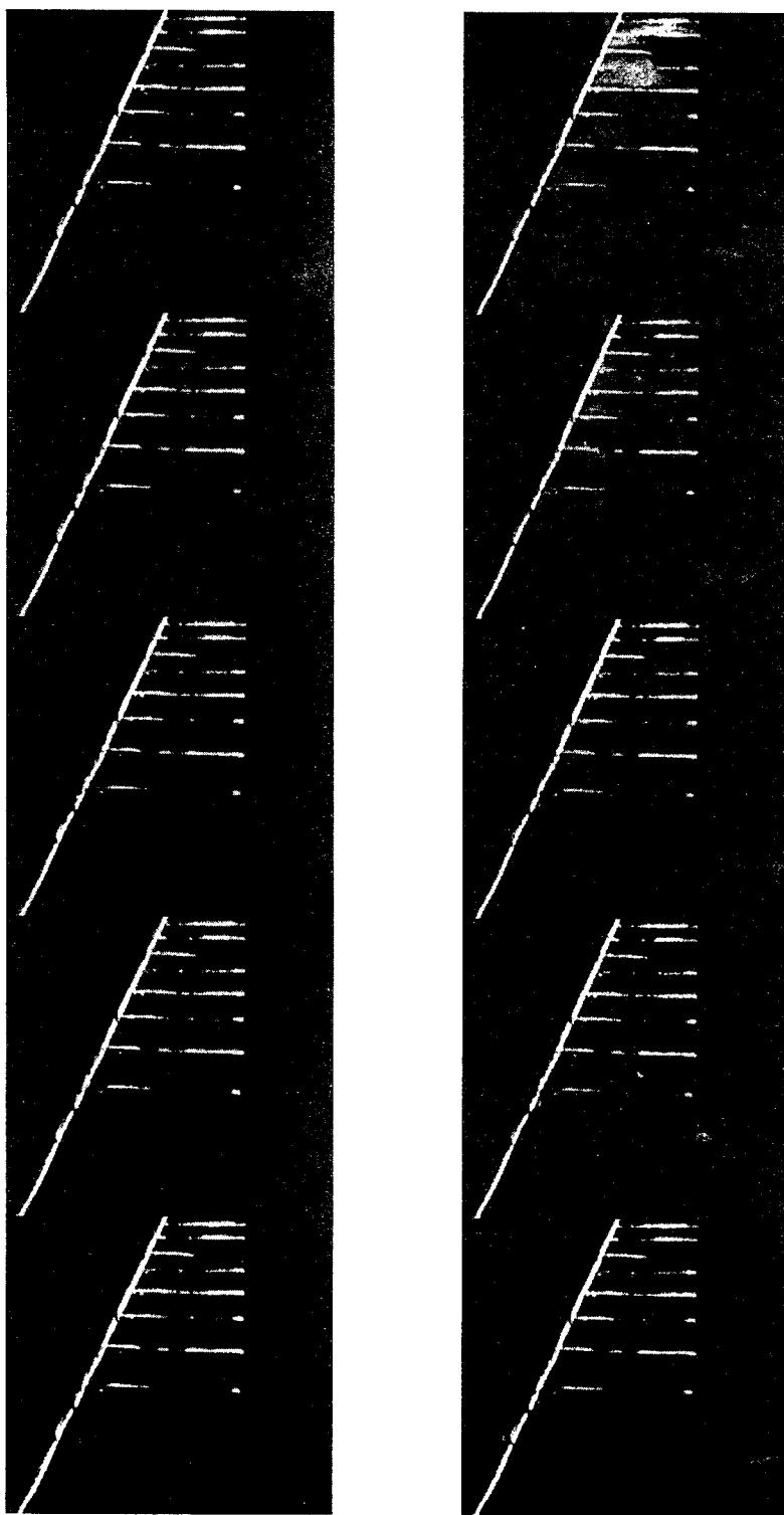
Fig. 3. The Development of a ceiling jet of 200mm pool fire
