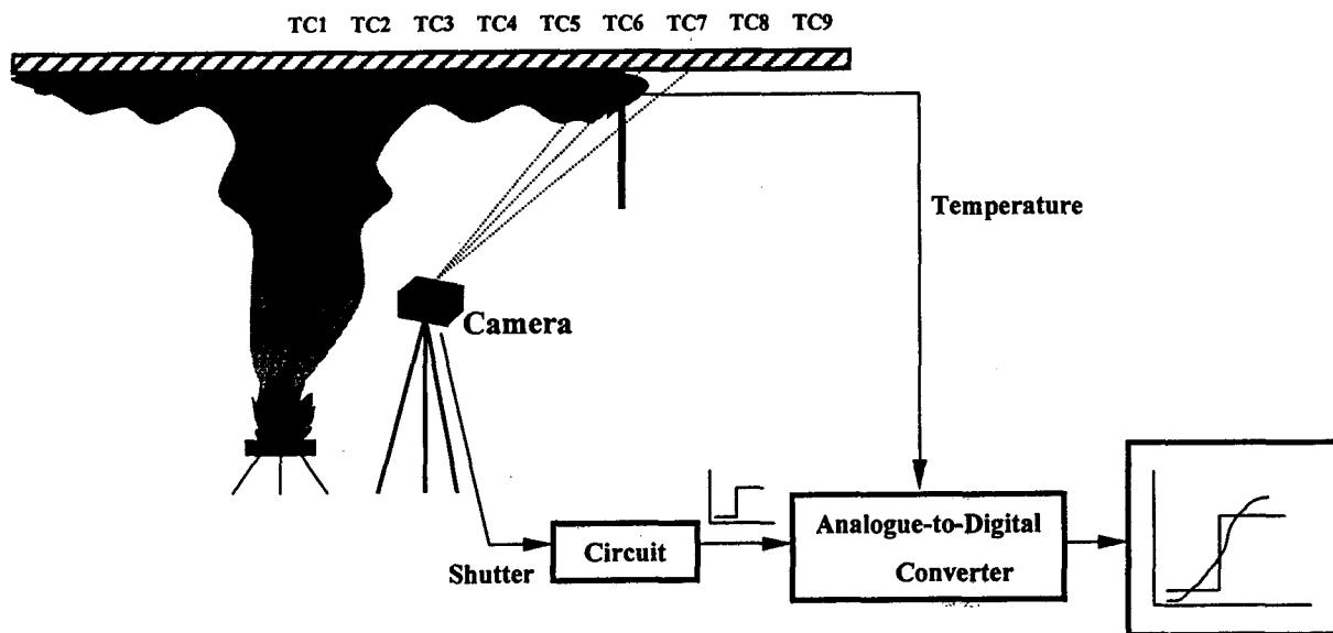
Fig. 2. The tracking of smoke front by a single-shot camera and thermocouples
