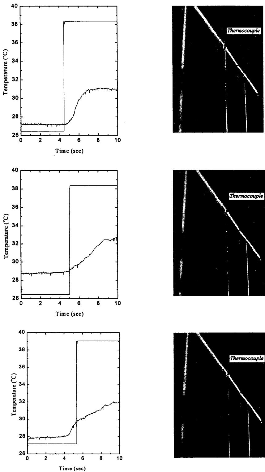
Fig 7. The synchronized smoke fronts with their temperature signals around TC6 (150mm pool fire)
