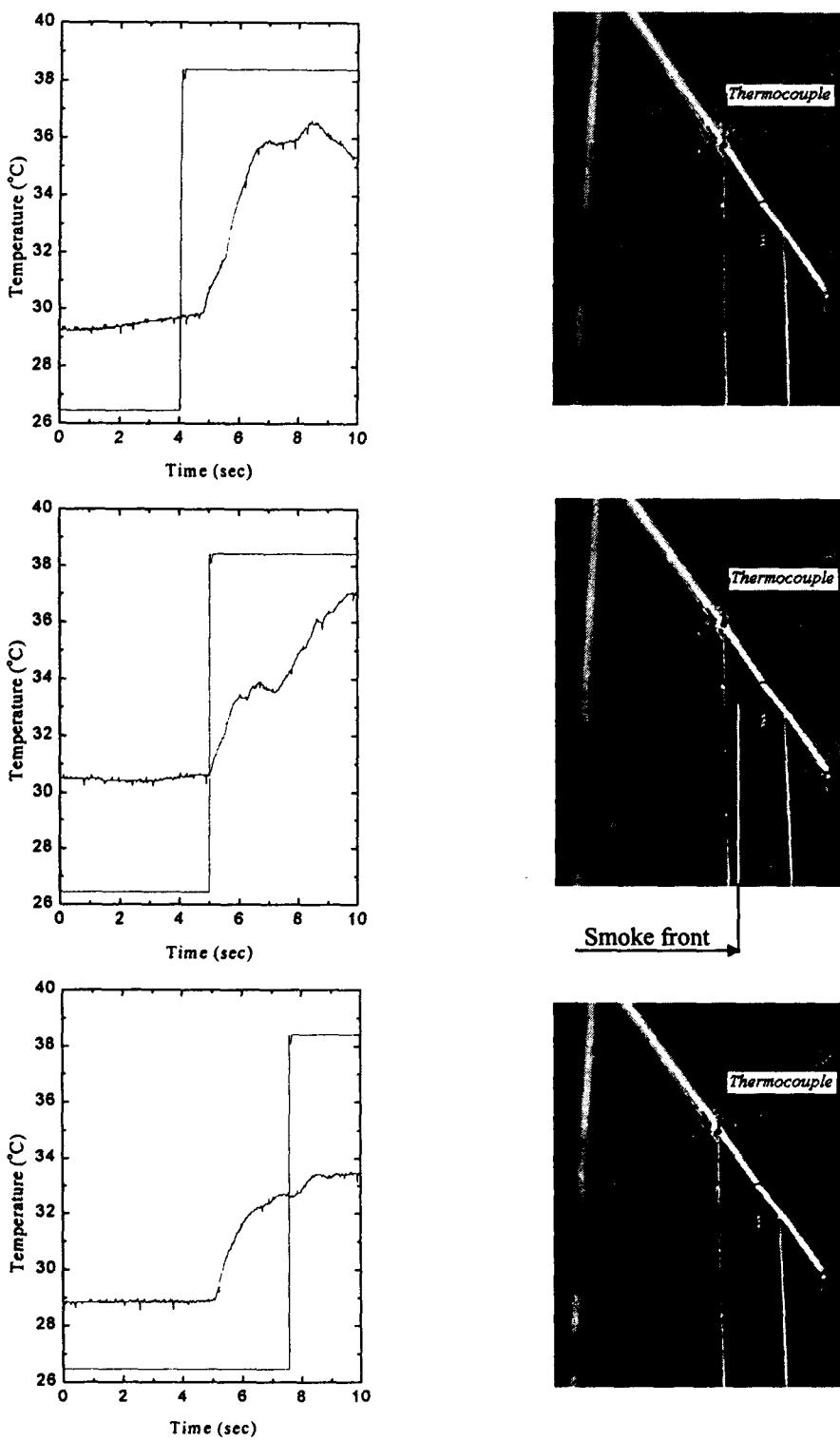
Fig 6. The synchronized smoke fronts with their temperature signals around TC6 (200mm pool fire)
