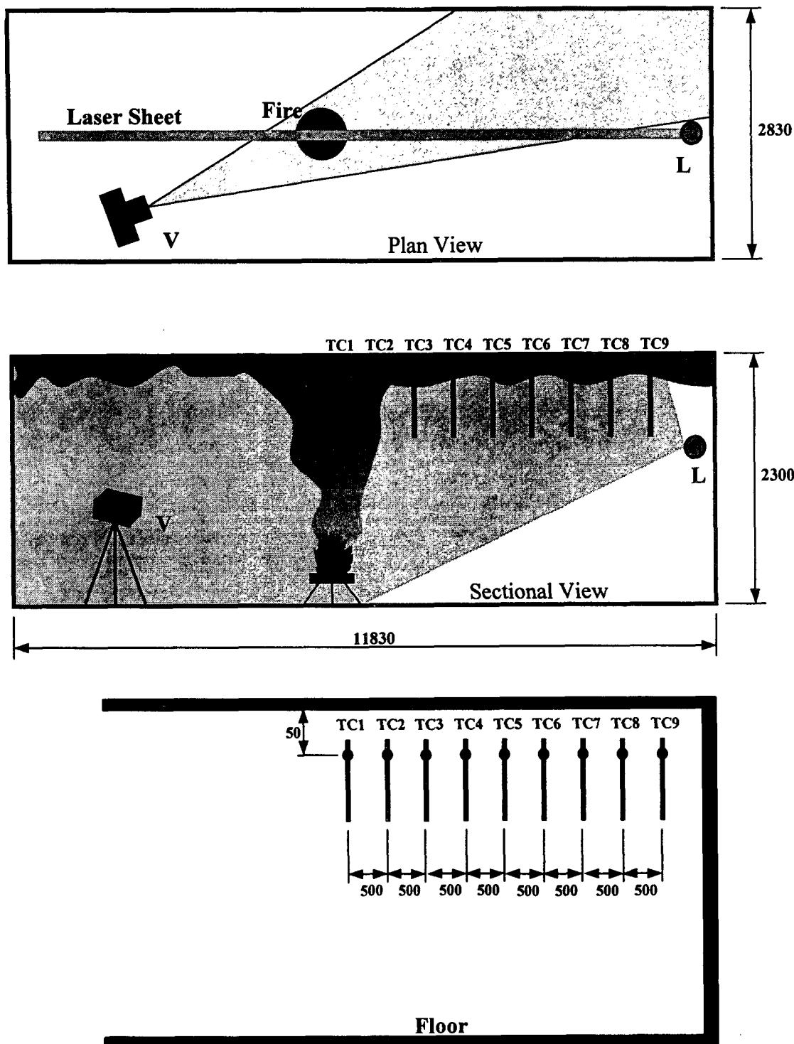
Fig. 1. A schematic diagram of the experimental apparatus
