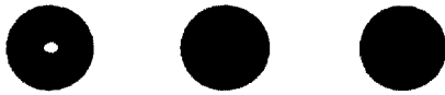
그림 18 Laboratory size concrete specimens used for the modeling. Cylindrical specimens with a 152.4 mm diameter with no inclusion, a 25.4 mm diameter rebar at the center, and a 25.4 mm diameter void at the center.
