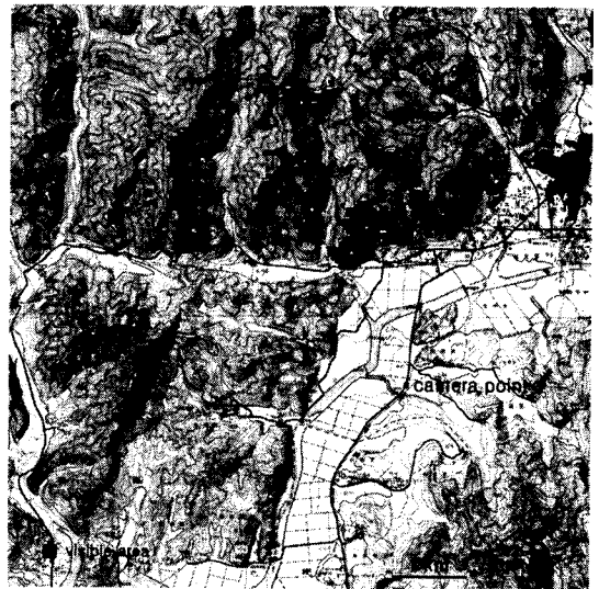
Figure 9. Visible area on topographic map from single camera point to view field.
