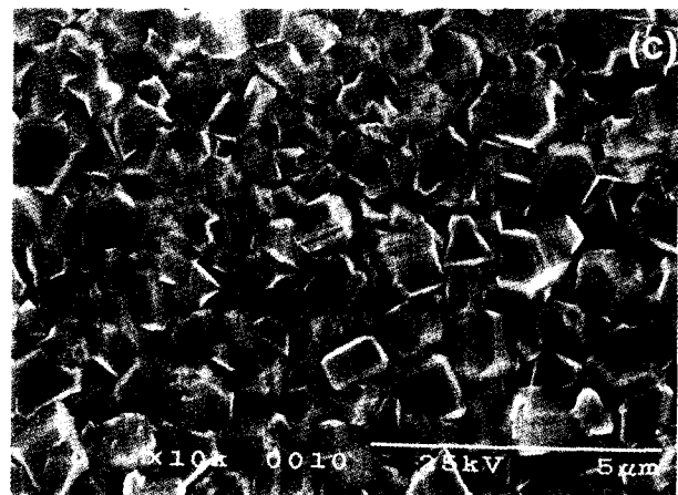
Fig. 3. SEM morphology of the diamond films deposited as function of the flow rate ratio of CO and H 2 mixture gases. (a) CO/H 2 = 0.11, (b) CO/H 2 = 0.18, and (c) CO/H 2 = 0.25.
