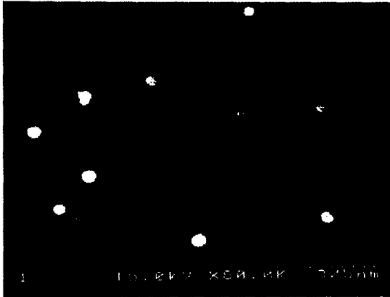
Fig. 3. SEM image of Cu particles on the initial Si substrate
