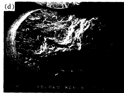
Fig. 5 SEM micrographs of fracture plane at 600°C (a) poly crystal( \times 50 ) (b) directionally solidified( \times 50 ) (c) <001> single crystal( \times 50 ) (d) <001> single crystal( \times 20 ).
