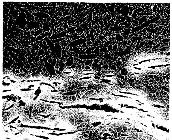
Fig. 1. SEM micrograph of \text{Si}_3\text{N}_4 coated \text{Si}_3\text{N}_4 -20wt%BN bilayer composite : top layer is coating layer, and bottom layer including BN phase(dark phase) is substrate layer.
