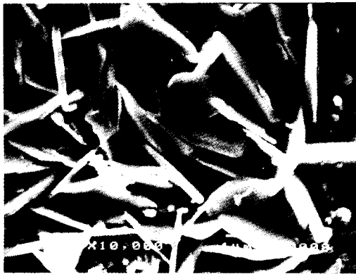
Fig. 3. SEM micrograph of the precipitate derived from kaolin.
