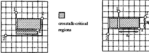
Fig. 1. Crosstalk and Crossing. Minimizing crosstalk may introduce more crossings.
