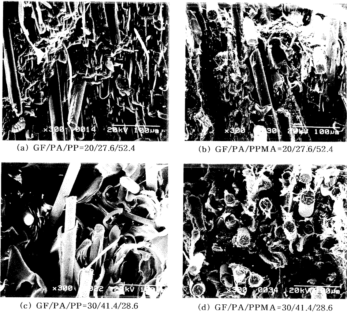
Fig. 3. Scanning electron micrographs for tensile fractured surface of GFPAPP and GFPAPPMA composites.
