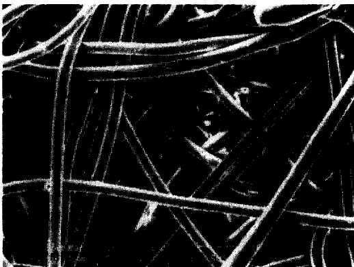
Fig. 1. SEM photograph of neutralized fabric filter.
