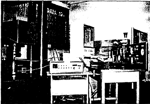
(b) Hydraulic test (Permeability tests with triaxial cell)
