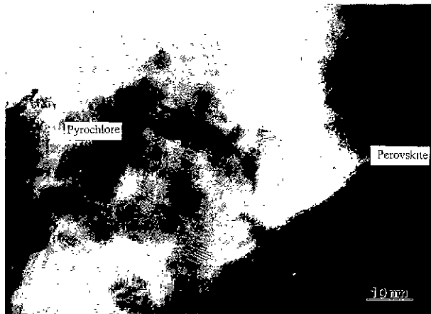
Fig. 7. HRTEM image of powder calcined at 650°C for 1 hour.
