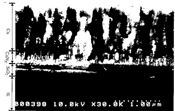
Fig. 5. Fracture cross-sectional morphology of the prepared Cu/CuN x /SiO 2 layer by SEM.
