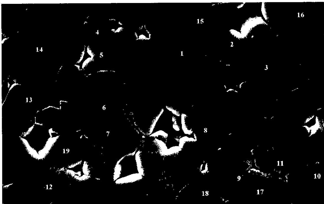
Fig. 4. The deformation twins in ZnO varistor sample of A-series with 1 wt% \text{Al}_2\text{O}_3 addition.
