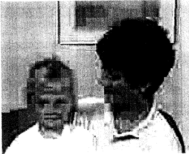
그림 6. Mother and Daughter sequence의 첫 번째 압축영상 (QP=25, PSNR: 28.13 dB) Fig. 6. Compressed 1st frame of Mother and Daughter sequence(QP=25, PSNR: 28.13 dB)
