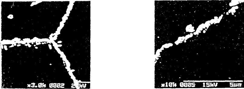
Photo 7. Intergranular Corrosion for Aging Heat Treated Specimen at 850°C × 16hrs.
