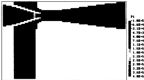
Fig. 9 Pressure distribution in water jet for location rear 1mm
