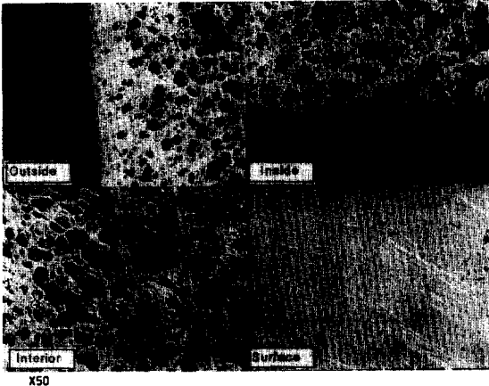
Fig. 11 Microphotograph of general pore distribution of trial manufactured diamond wheel
