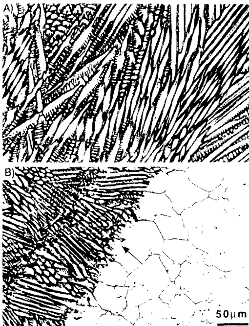
Fig. 10 Micrographs of GTA weld in type 309S stainless steel: A) center; B) fusion boundary
