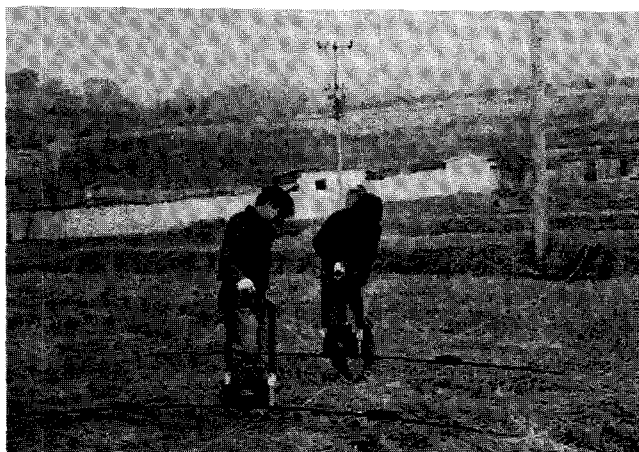
Pic. 3. Field data acquisition with GPR method (pulseEKKO IV).
