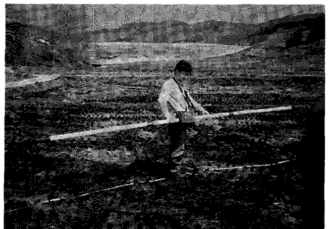
Pic. 2. Field data acquisition with electromagnetic method (EM 31).
