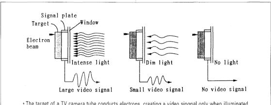
\* The target of a TV camera tube conducts electrons, creating a video singnal only when illuminated.
