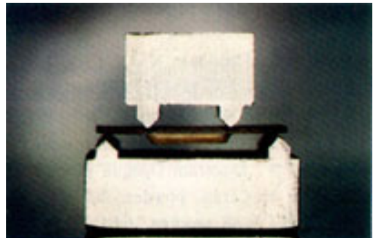
Fig. 4. Four point flexural test arrangement. Upper two load points were 14mm apart and the distance between two lower supports was 23mm.
