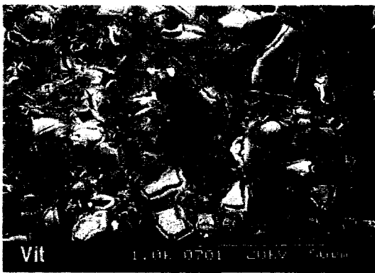
Fig.9. Etched structure of Vitremer (x1000).
