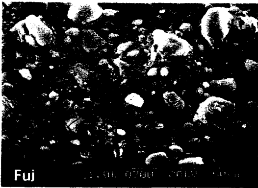
Fig.8. Etched structure of Fuji Duet (x1000).
