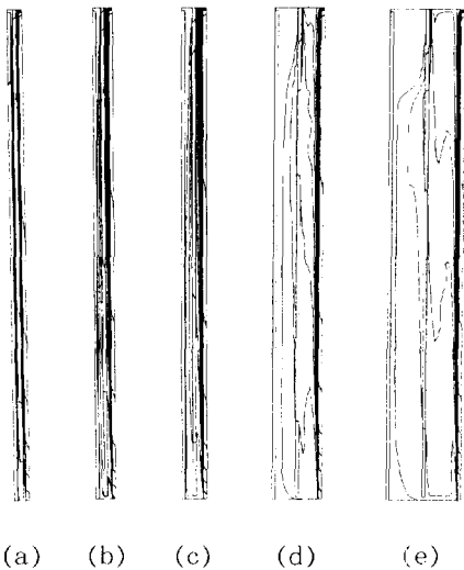
Fig.6 Isotherms for I_s=10W/m^2 and Re=300 at various aspect ratios; (a) W/H=0.03 ( \theta_{max}=0.517, \theta_{min}=0 ), (b) W/H=0.04 ( \theta_{max}=0.601, \theta_{min}=0 ), (c) W/H=0.05 ( \theta_{max}=0.636, \theta_{min}=0 ), (d) W/H=0.1 ( \theta_{max}=0.640, \theta_{min}=0 ), (e) W/H=0.15 ( \theta_{max}=0.640, \theta_{min}=0 )
