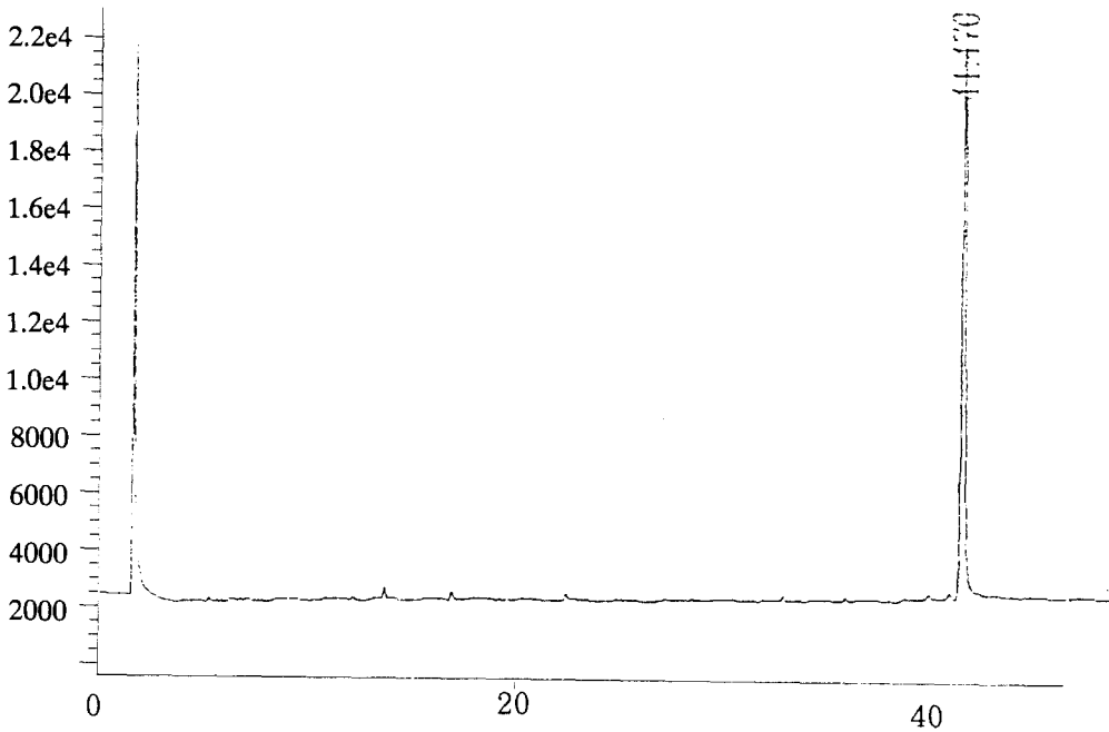
Fig 2. Gas chromatogram of acetonitrile extracted blank control beef fat *. Ret. time 41.470 is internal standard(dibutylchloredate)
