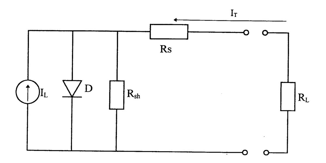
Fig. 1. Equivalent circuit of a solar cell
