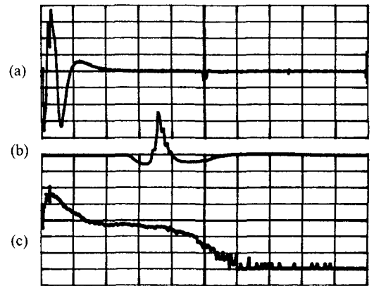
Fig. 4. (a) Full range signal (hor. : 2 μs/div., ver. : linear) (b) The first echo obtained by reflection testing for the top surface of a specimen at the distance of 7.4mm from the PVDF transducer (hor. : 50ns/div., ver.: linear) (c) Frequency spectrum of the echo (hor. : 20 MHz/div., ver. : 20dB/div.).
