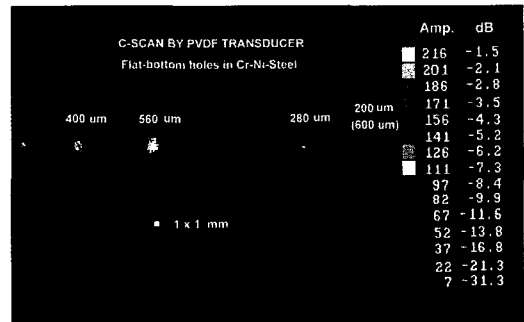
Fig. 8. C-scan image for the fine grained Cr-Ni steel with flat-bottom holes of diameter 400 \mu m, 560 \mu m, 280 \mu m and 200 \mu m positioned at 12mm depth, where only the hole of diameter 200 \mu m was drilled from the pre-drill hole of diameter 600 \mu m at 13.4mm depth.
