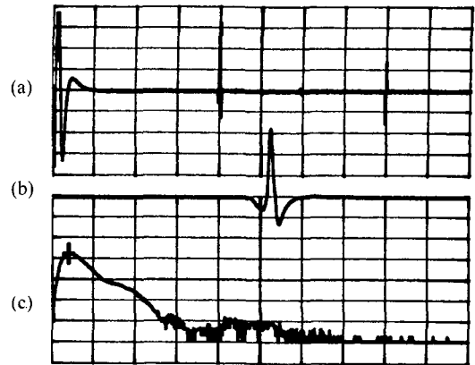
Fig 3. (a) Full range signal (hor. : 5 μs/div., ver. : linear) (b) The first echo obtained by reflection testing for the top surface of a specimen at the distance of 14.8mm from the PVDF transducer (hor. : 100ns/div., ver.: linear) (c) Frequency spectrum of the echo (hor. : 20 MHz/div., ver. : 20dB/div.).
