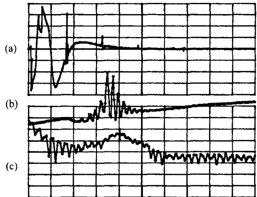
Fig. 6. (a) Full range signal (hor. : 1\mu\text{s}/\text{div.} , ver. : linear) (b) The first echo obtained by reflection testing for the top surface of a specimen at the distance of 1.3mm from the PVDF transducer(hor. : 50\text{ns}/\text{div.} , ver. : linear) (c) Frequency spectrum of the echo (hor. : 20 MHz/div., ver. : 20dB/div.).
