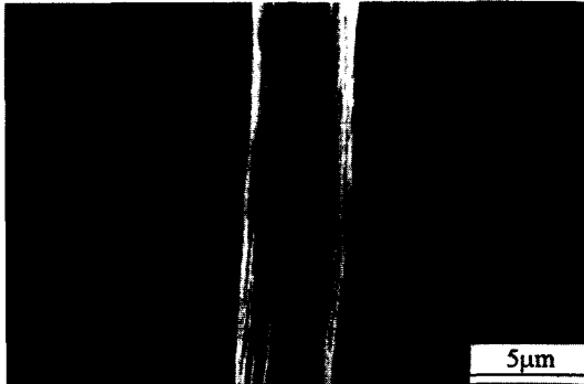
Figure 10. Scanning electron micrograph of in-situ pulped PVA fiber.
