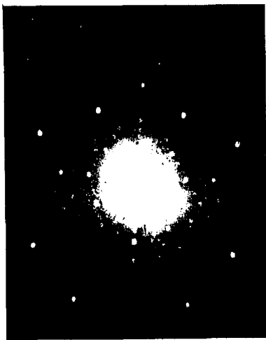
Fig. 4. A laue X-ray back-reflection photograph of the LiTaO 3 crystal grown in the Y-axis orientation.
