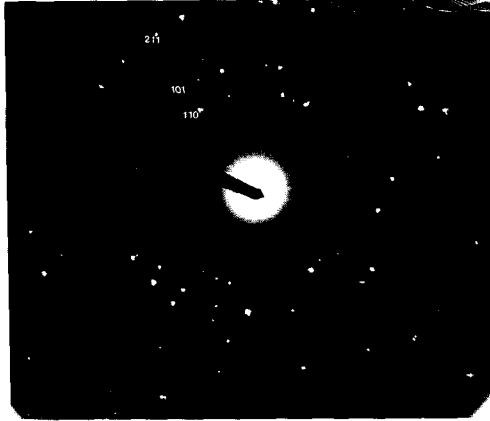
Fig. 5. Electron diffraction pattern of a Pt/SnO 2 .
