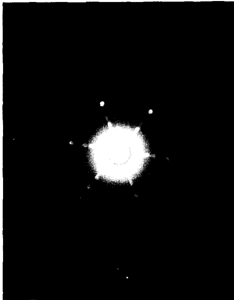
Fig. 3. X-ray Laue pattern from the top surface of the 6H-SiC single crystal, showing the 6-fold symmetry.
