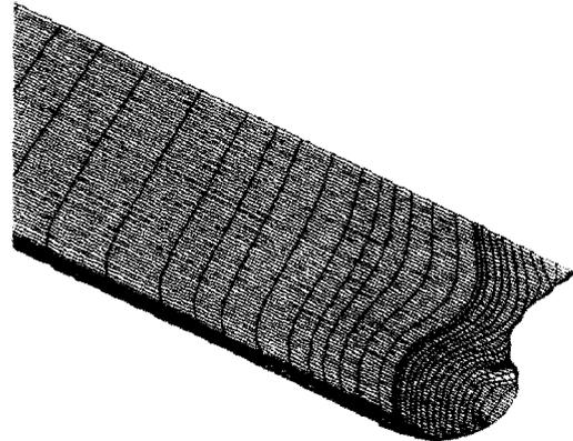
Fig. 7. The result of actual hullform design of ship (fore-body).
