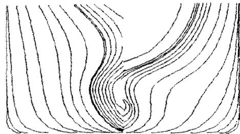
Fig. 8. The result of actual hullform design of ship (body plan).
