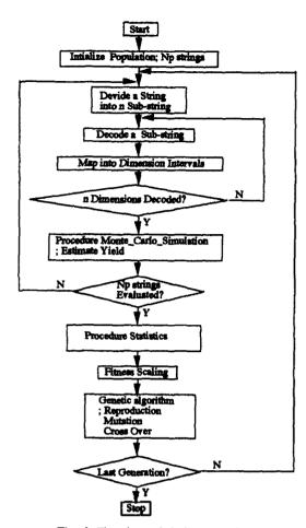
Fig. 4. Flowchart of design centering.
