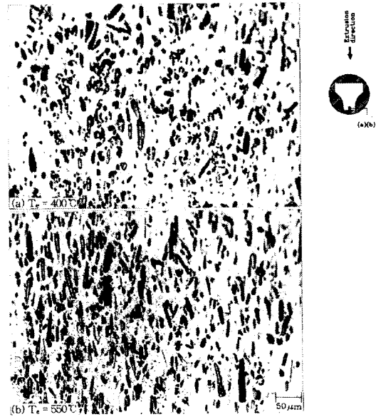
Fig. 7 Microstructure of fiber orientation on middle portion of die exit depending on extrusion temperatures at extrusion ratio, 8.5 (100 \mu m)
