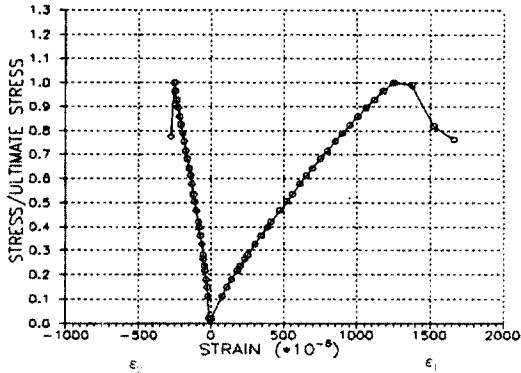
Fig. 5 Stress-strain curve (pore ratio=0.61)
