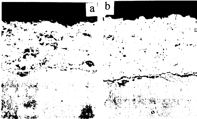
Fig. 9. Microstructure of coatings with different deposition efficiency (200×) (a) 24% and (b) 57%
