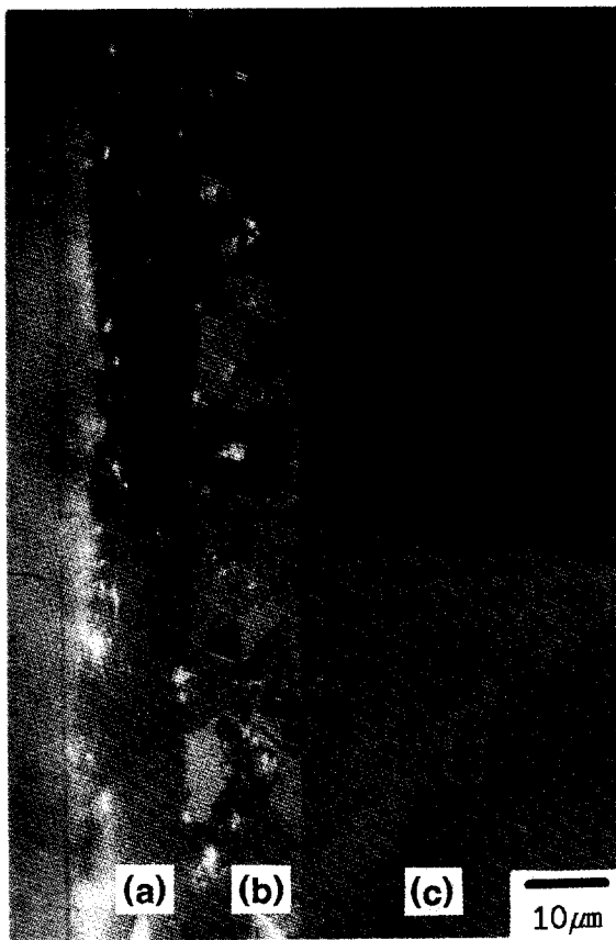
Photo 2. Layer of nitride material formed from CVD. (a) \delta -TiN 1-x (b) \epsilon -Ti 2 N (c) \alpha -TiN
