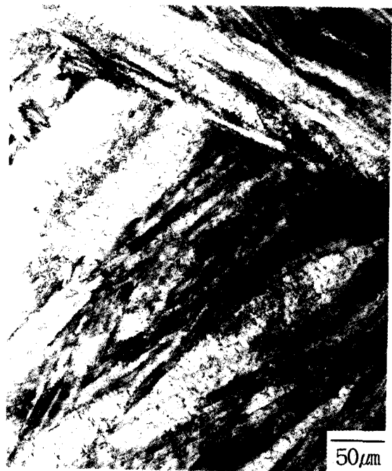
Fig. 2. Microstructure of oil quenched 0.58wt.% Mo added steel.
