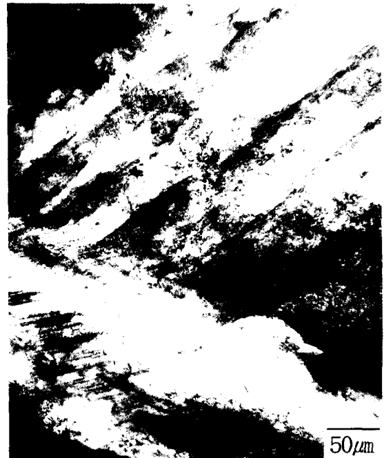
Fig. 1. Microstructure of oil quenched 0.30wt.% Mo added steel.
