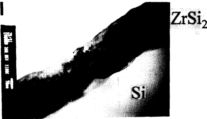
Fig. 4. TEM micrograph of the Zr/Si thin film after annealing at 800°C
