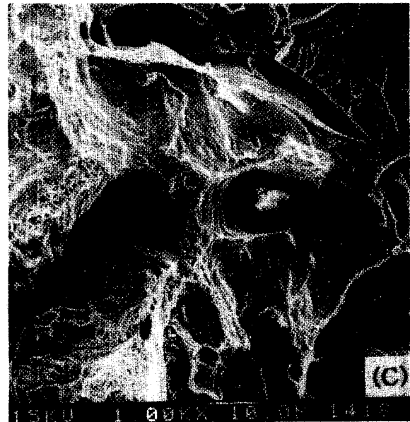
Fig. 11. SEM fractographs of cast CF-8M stainless steel(specimen "C") after aging at 400°C, 2,000 h and charpy impact failure at 25°C. (A) overall fracture surface; (B) and (C) higher magnifications of (A), showing ductile and brittle-cleavage morphology
