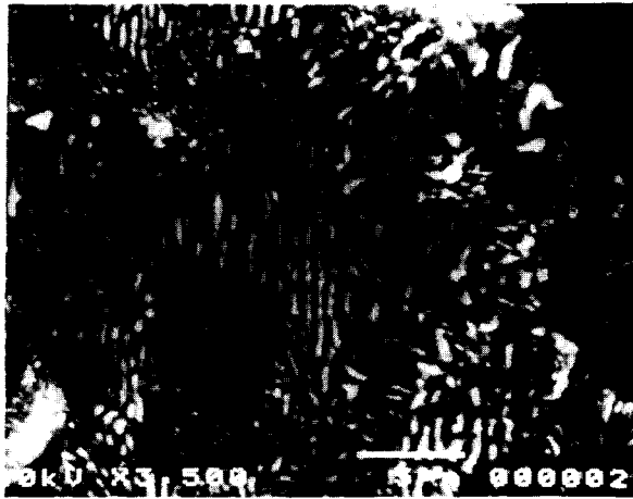
Fig. 9. SEM micrograph of Mg-9Al-2Zn alloy aged at 200°C for 72hrs.(over aged condition)
