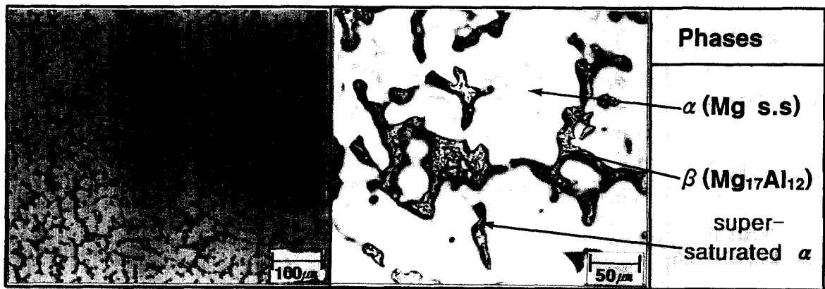
Fig. 4. Optical micrographs of as squeeze cast Mg-9Al-2Zn alloy.
