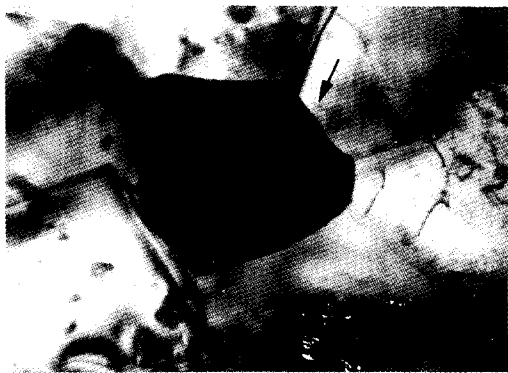
(b) Al_3(Ti+Ce) in Al-8Wt.%(3Ti+1Ce) alloy
