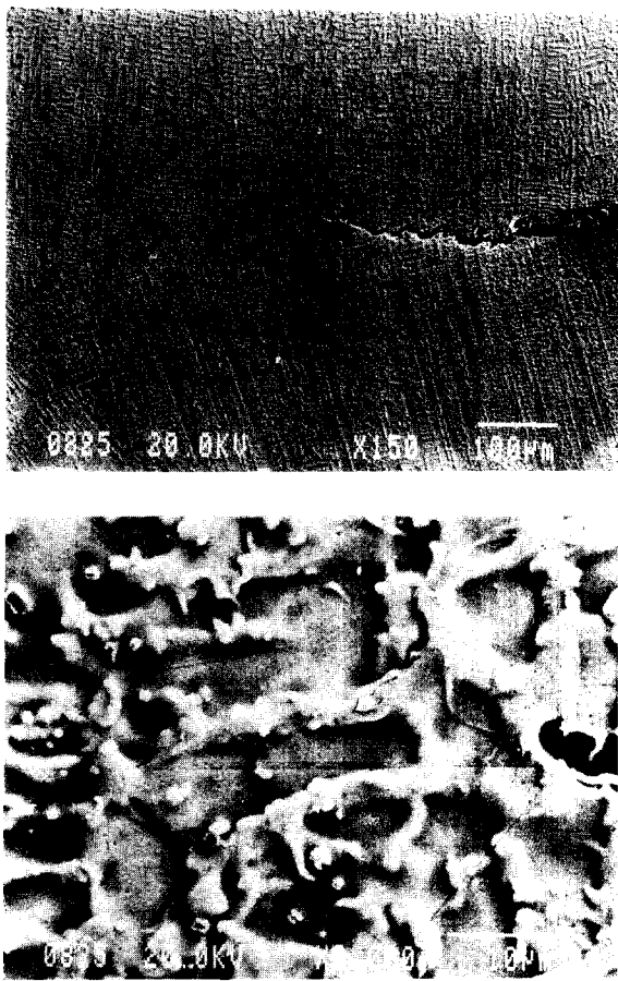
Fig. 9. Typical centerline crack in weld of 825-SS41-Inco112.
